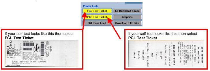
14. Once the Test Ticket selection box comes up, click on the Send button to print out a ticket. You will see one of the two below depending which test you selected in step 11.
